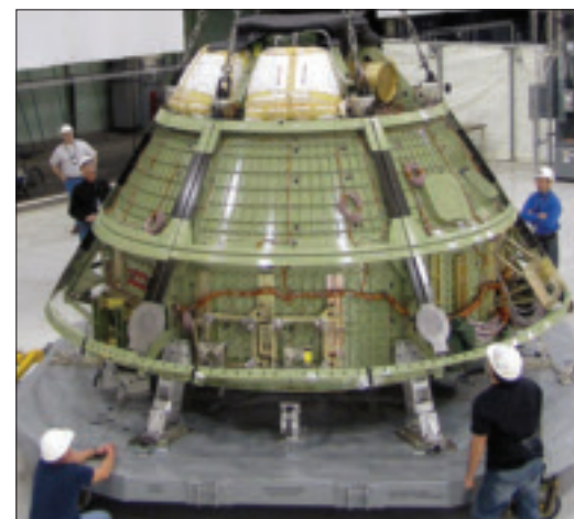
The Orion crew module ground test structure is inspected prior to integration with an encapsulating aeroshell. The NASA administrator believes work on the Orion CEV can be integrated with development of an MPCV.
